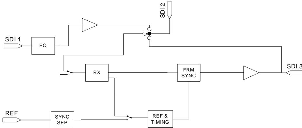
This diagram shows how the video flows through the V1643. In particular the selection for SDI 2 between a second input, a buffered output and a main output can be seen. This drawing is diagrammatic and should not be read literally; for example it may seem that there is no equaliser (EQ) for SDI 2 when it is being used as an input but this is not the case since in fact the EQ is inside the Receiver block (RX) along with the selection switch.
