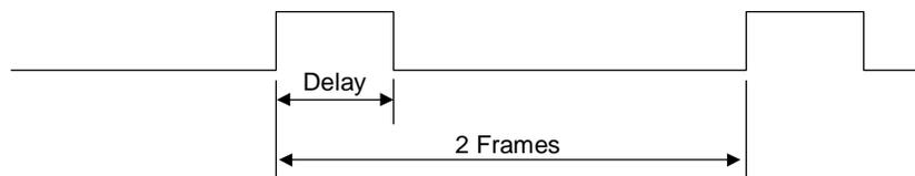
If the unit is not synchronising, such as loss of i/p or Freeze then the delay output is blanked. It is expected under these conditions that the audio processing will hold its current delay from the last valid measurement until a pulse re-appears. This is what the internal audio delay does.
