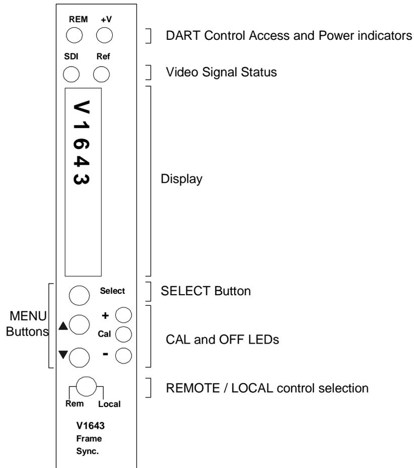
The front panel on the V1643 is a considerable advance on what is usually available on single module interface equipment. It provides the user with total control and monitoring of the unit without the need to consult manuals and read unlabelled indications. While this kind of control is generally available with a remote control system, as it is over DART, it is unusual to have this level of access locally.
